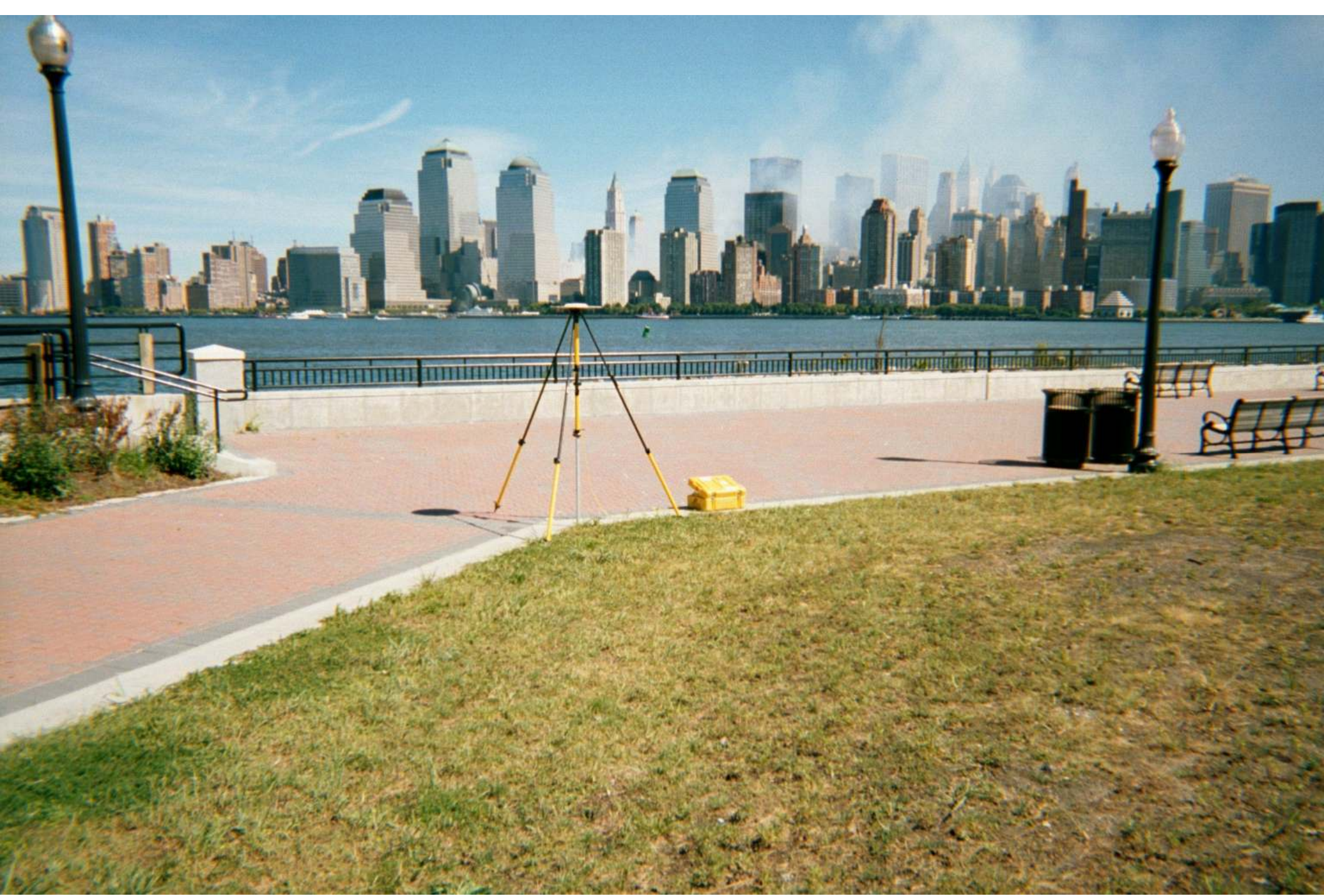
NOAA/NGS GPS Receiver at Liberty State Park, NJ supporting the collection of airborne LIDAR and Photography over the WTC site.
