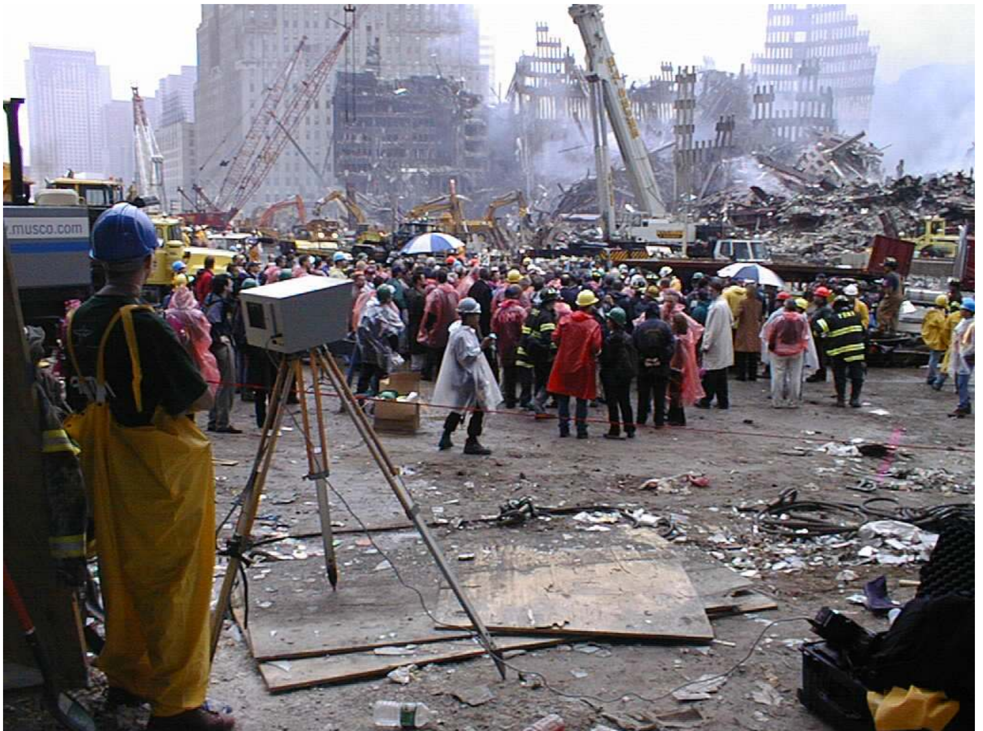
Optech employee and ground LIDAR working at WTC
